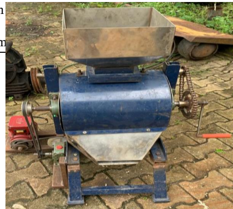
Figure 3. The developed cowpea bean seed dehuller.
