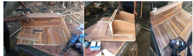
Figure 8. Fabrication Process of the Master Jig
