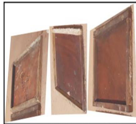
FIGURE 10: Wooden Moulds for Manufacturing of Board
