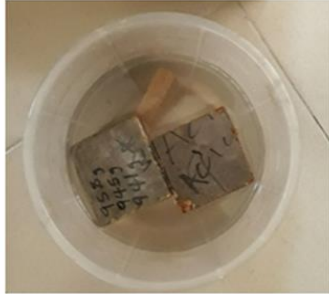
Plate 1: Dipping During Thickness Swelling and Absorption Test.
