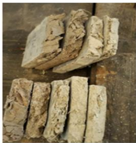
Plate 2: The Board Samples after Compression Test
